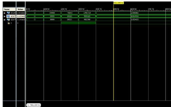
**Figure 12. Simulation Output Of 128 Bit Adder**
