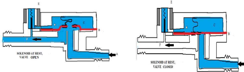
**Figure 1.6** Working of Solenoid valve
