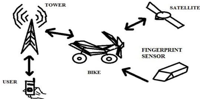
*Figure 1.7 Overall view of bike security system*
