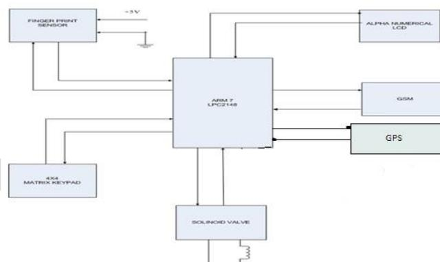
Figure 1.2 Block Diagram of security system
