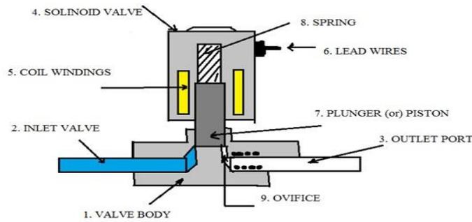
**Figure 1.5** Parts of Solenoid Valve
