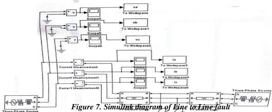
Figure 7. Simulink diagram of Line to Line fault
