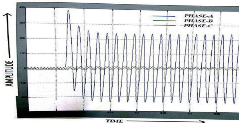
Figure 6. Output currents waveform for Single Line to Ground Fault
