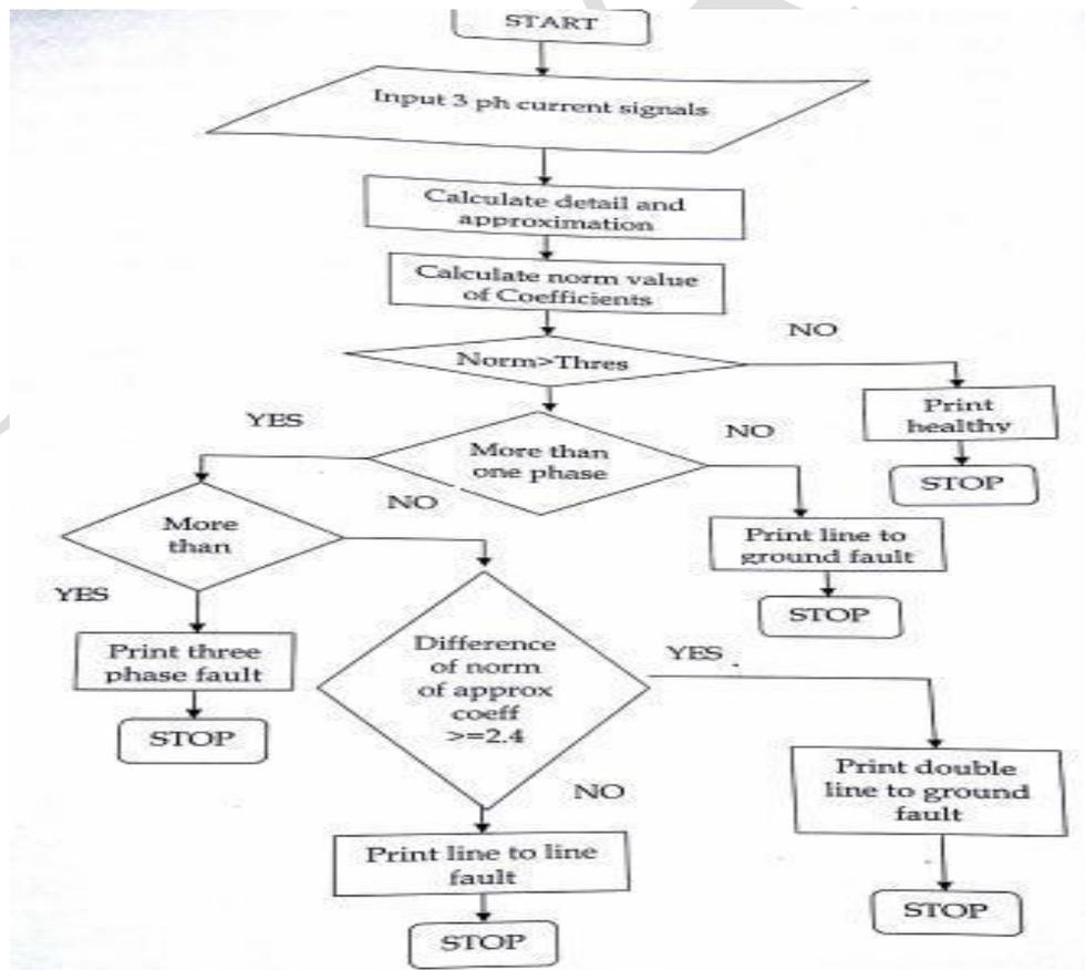
Figure 4. Fault classification algorithm
