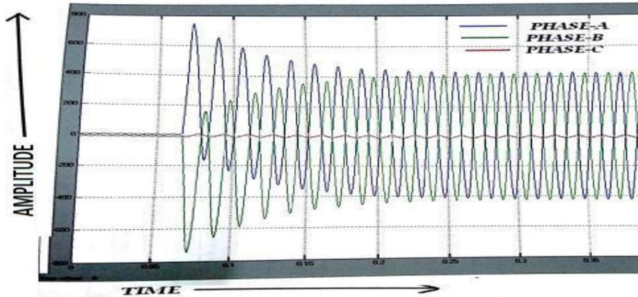
Figure 8. Output currents waveform for Line to line Fault
