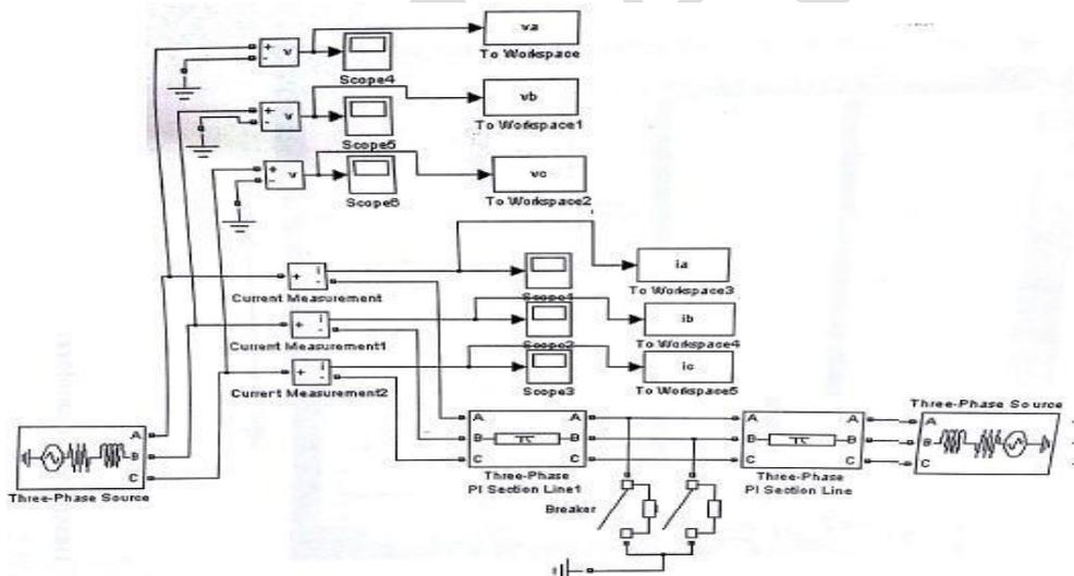
Figure 9. Simulink diagram of Double Line to Ground fault
