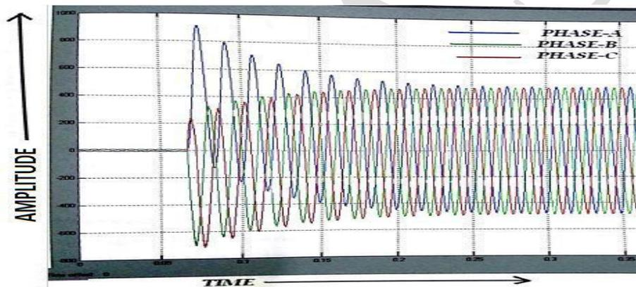
Figure 12. Output currents waveform for Three phase Fault
